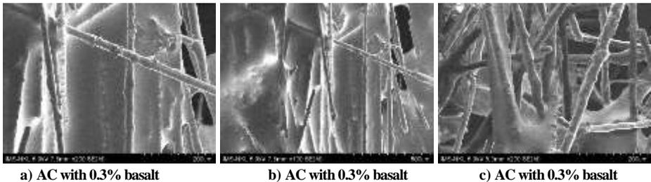
Fig. 2.8. Bonding between basalt fibers in the asphalt mixture
