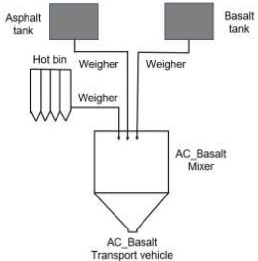
Fig. 4.7. Production of basalt fiber AC at the mixing plant
