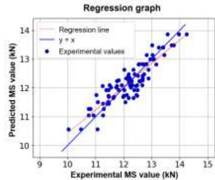
Fig. 4.2. Regression graph showing the prediction results by XGB model.
