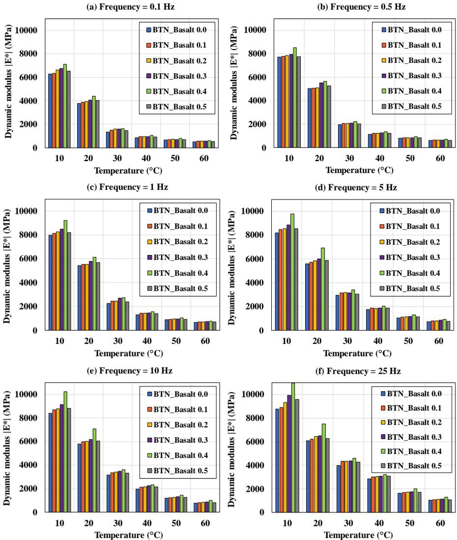
Fig. 3.26. Influence of the temperature to  $|E^*|$  of 6 types of AC.
