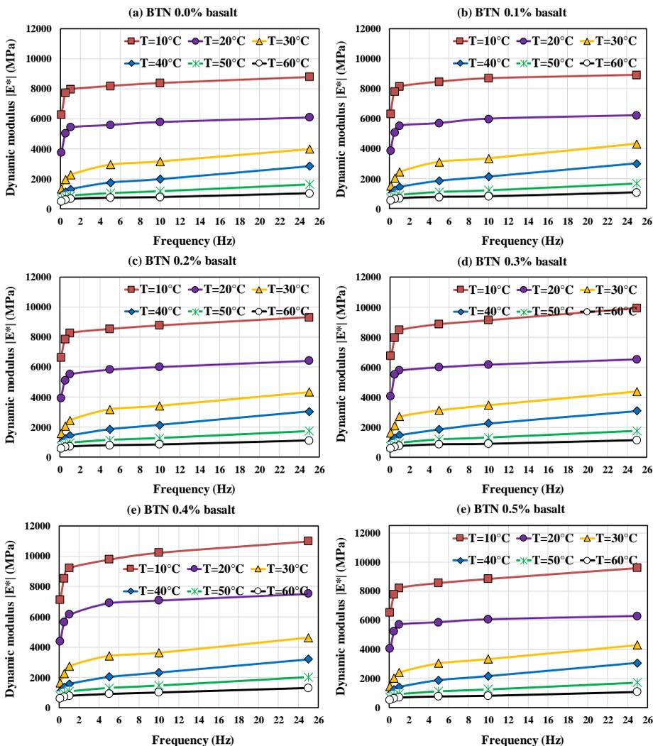
Fig. 3.25. Influence of the frequency to  $|E^*|$  of 6 types of AC.
