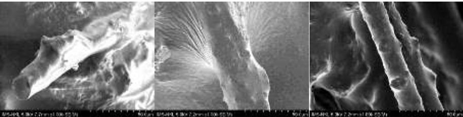
Fig. 2.6. Bonding between basalt fiber and binder.
