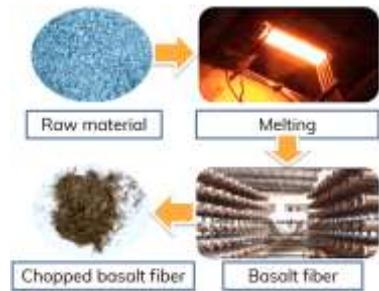
Fig. 1.2. Basalt fiber production process.
